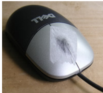
Figure 4.4 Traditional mouse with disabled scroll wheel
