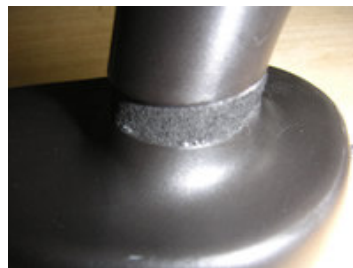
Figure 4.6 Foamed rubber at basis of the Sico mouse
